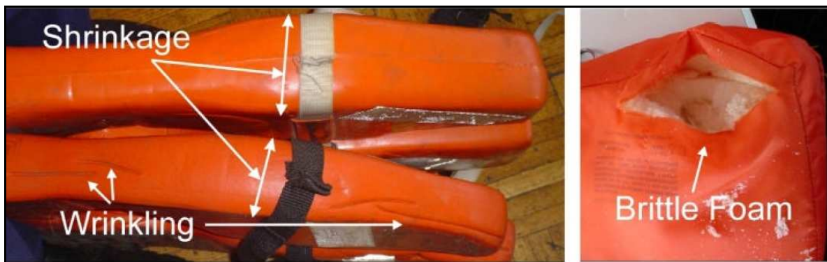
Left image shows an example of a vinyl dipped PFD with compressed or hardened foam. Right image illustrates a fabric covered PFD with brittle foam.
